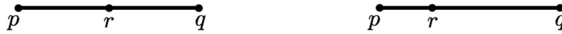
FIG. 2. The new node on an edge pq (left – right): p \neq Q and q \neq Q (midpoint); p = Q ( |pr| = \kappa|pq| , \kappa < 0.5 ).
